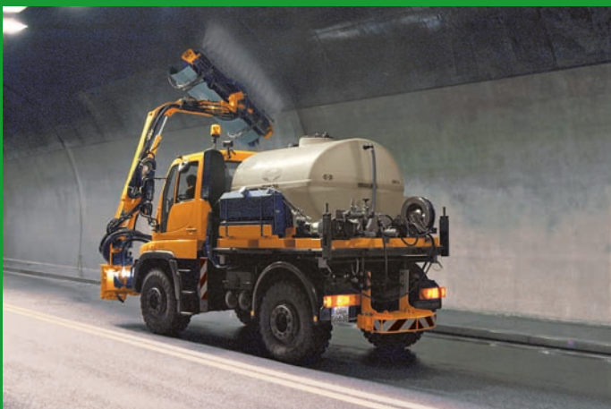
Automatic adaption of the washing brush to the wall
